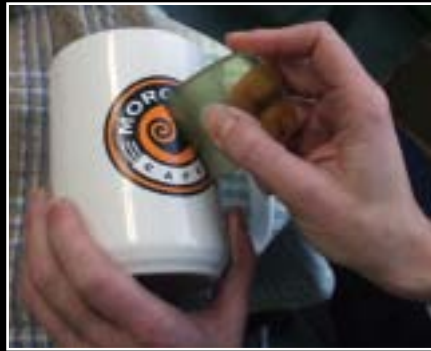
A squeegee is used to remove any water and air bubbles.
