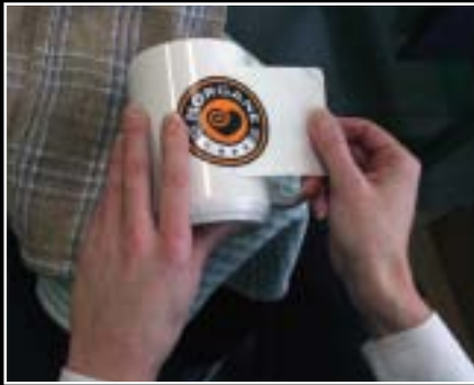
The color print is dragged from the decal paper to the ceramic or glass surface to decorate.
