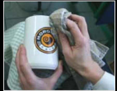
Excess water is removed, and the piece is allowed to dry at room temperature for one day.
